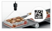
Two or more different codes in the same field of view can be read by utilizing a high resolution camera. This function helps to reduce the inspection time.
